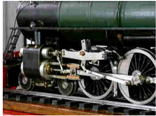
Piston valves, Cylinders and Transmission
